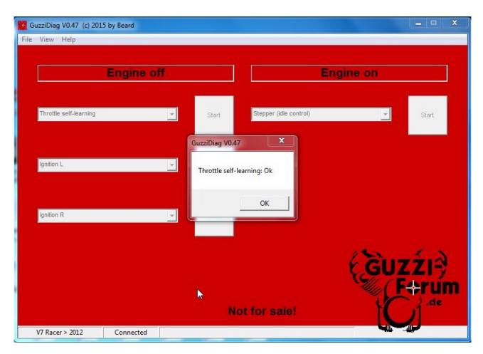
To reset the autolearning parameters, select 'Reset autolearning parameters' from the drop-down menu. Click 'Start', then 'OK'.
