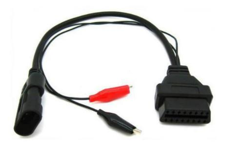
To connect to the bike, connect the two 16 pin connectors on the cables together and the 3 pin cable to the diagnostic port. It is usually tucked down beside the airbox. The diagnostic port only has two wires.
