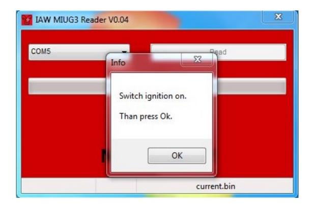
Turn your keyswitch to 'on'. Do not start the engine. Reader will start downloading. It will take 15 minutes to backup the map. It does not delete the map in the ECU. The Reader will also write a plain text file with the map details. I recommend you keep this with your saved map.
