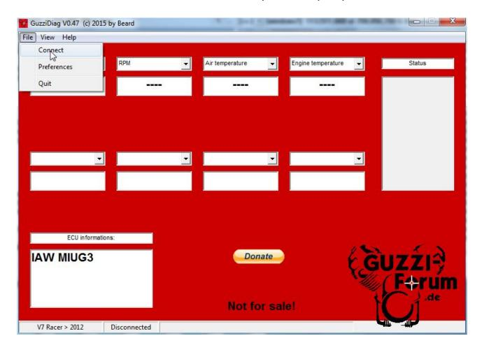
Select values to read from the drop down boxes. Here I have chosen 'Throttle', 'RPM', 'Air temperature' and 'Engine temperature'. When loading a new map, always make sure that 'Throttle' is one of the values'.
