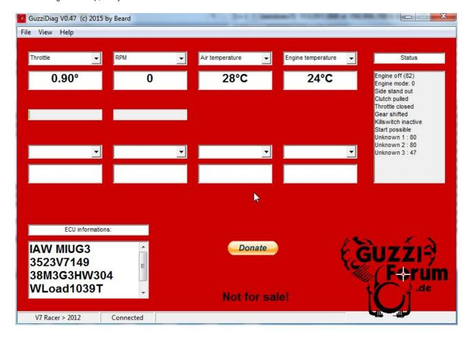
Here, you can see that after loading a map, the throttle value is 0.00. For a V7I & V9 it should 0.9 - 1.0. For a V7II, 1.0 - 1.2. For V7III, 0.8 - 1.0
