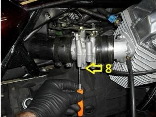
Once these are closed, remove the screws from the inlet manifolds (or disconnected the hoses for the charcoal can on US bikes) and connect your manometer (or balance tool).
